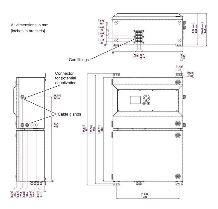
Fig. 2-9: X-STREAM XXF - Dimensions
